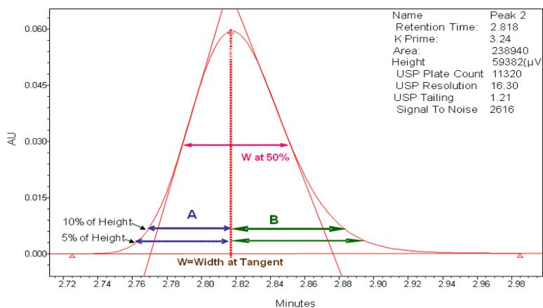
Figure 5: System Suitability measurements on a single peak
